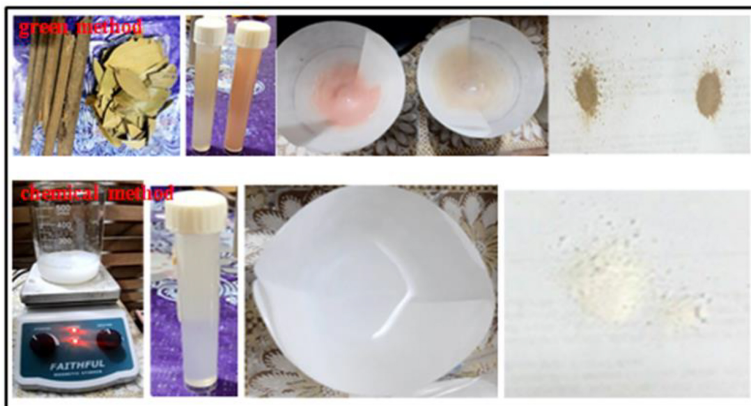
Fig. 1. Process steps for preparing ZnO NPs by chemical and green methods.
