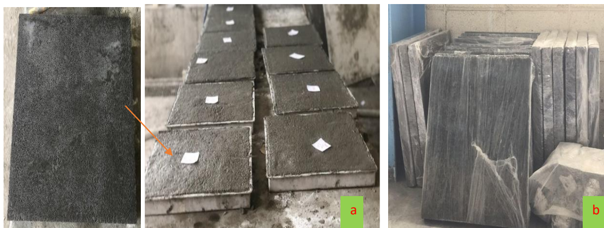
Figure 3: a-Samples of foamed concrete tiles into plastic molds. b- Curing foamed concrete tiles by wrapping them in plastic film
