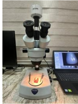
Figure(2) : Evaluation of surface of specimens by stereomicroscope.
