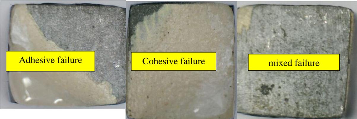
Fig. 2: demonstrates the specimens' CO-CR surface following their de-bonding from the ceramic during the shear bond strength test.
