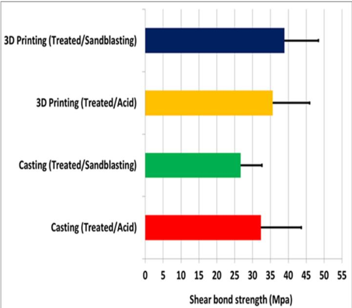
Fig. 3: Bar graph displaying the study groups' mean distribution of shear bond strength (SBS)
