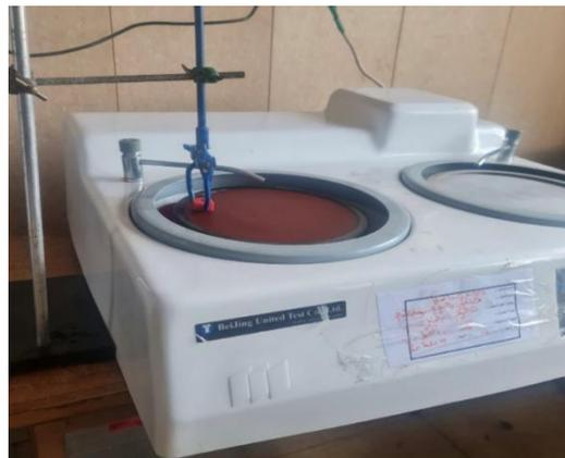
**Figure 4.** The polisher machine with the ceramic sample was fixed in its place using a metal holder.
