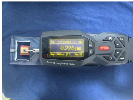
**Figure 5.** Surface roughness measurements of the samples with a 2D profilometer.
