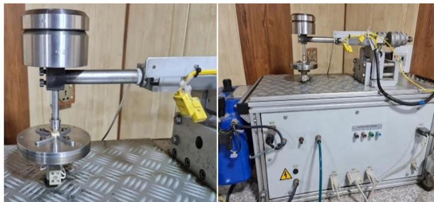
**Figure 6.** Pin on disc wear device and the sample was fixed at the cylindrical platform.
