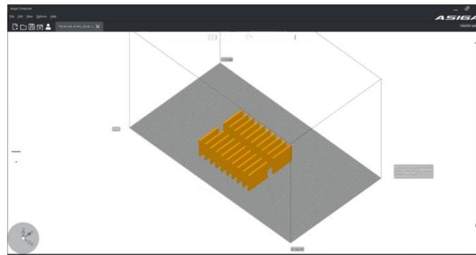
Figure 2. Design of 3D printing samples with Max UV (version 385) program.
