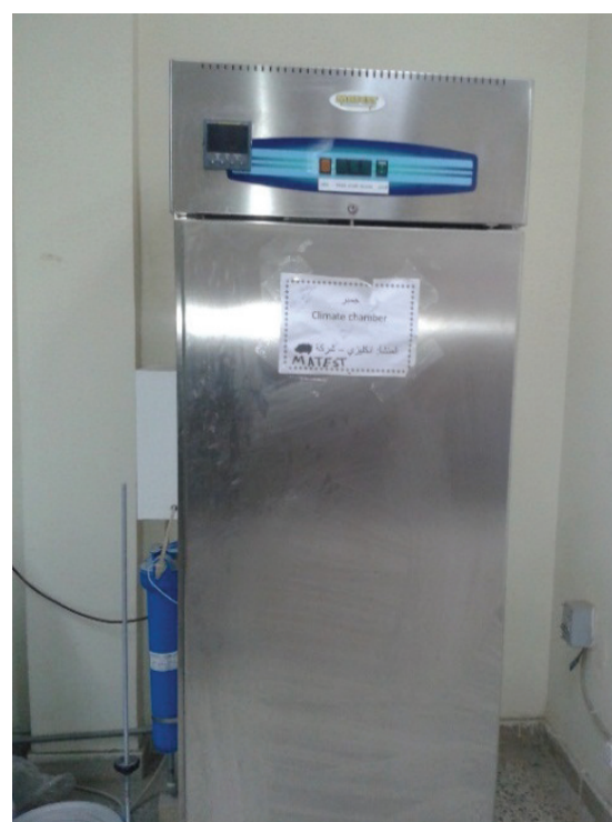
Plate (1): experimental setup: (a) freeze-thaw climatic chamber in the University of Technology.
