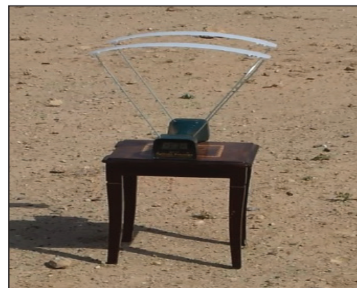
Fig. (3): The ballistic chronograph
