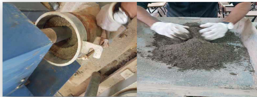
Fig. 2. Compaction process of soil.
