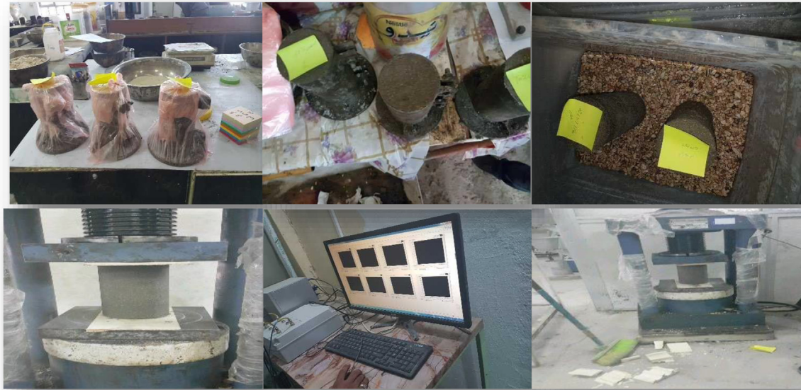
Fig. 6. Unconfined Compressive strength test.
