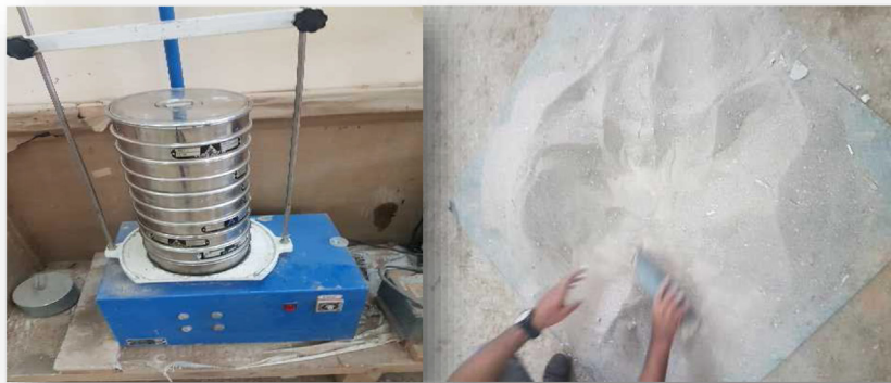
Fig. 1. Quartering and electrical sieving.
