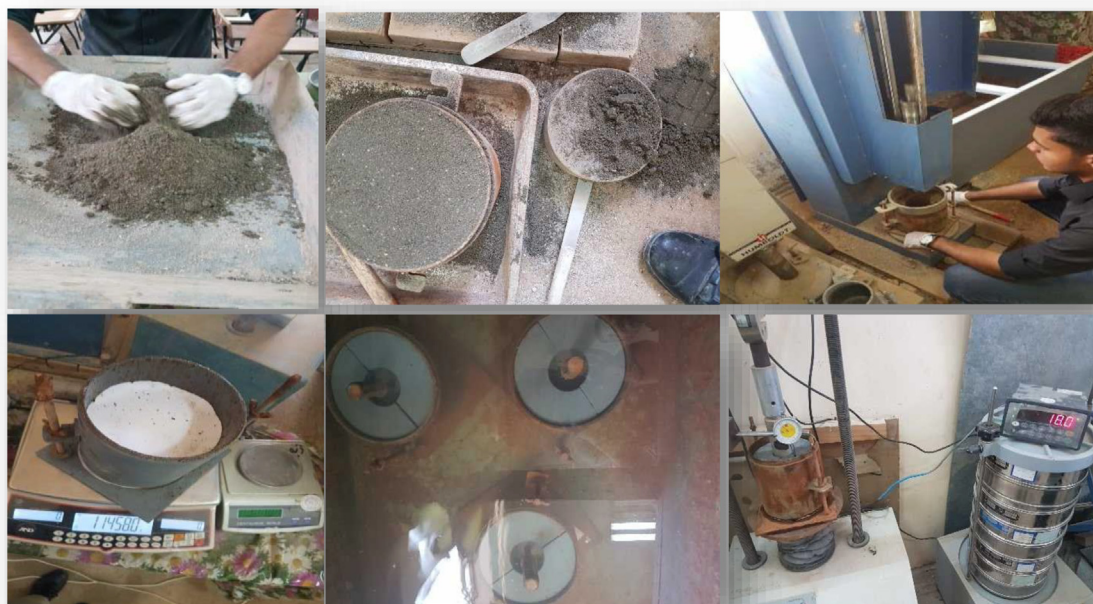
Fig. 4. Procedure of CBR % test.
