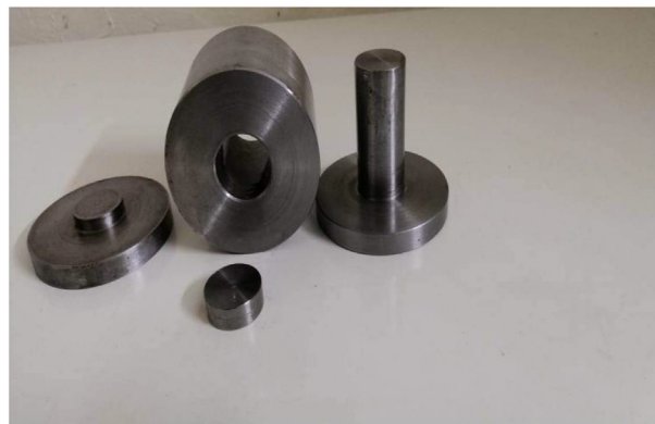
Fig. 1. The die used to press with a diameter of 10 mm.
