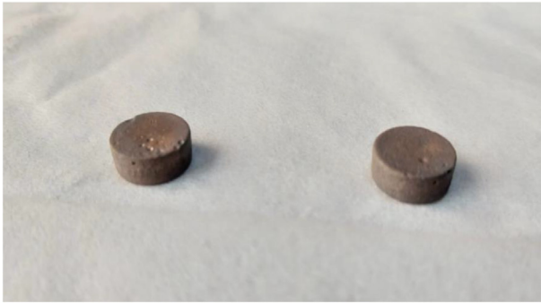
Fig. 2. Samples obtained from 15% compression after thermal sintering.
