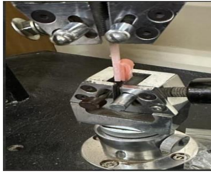
Fig. 6. Peel bond test by universal testing machine
