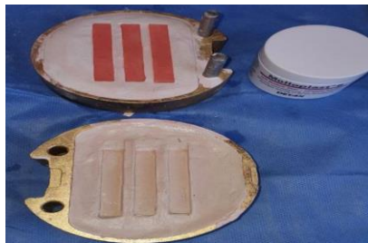
Fig. 4. The flask-containing acrylic resin specimens with wax patterns covering
