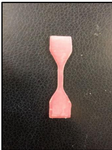
Fig. 3. Sample after polishing
