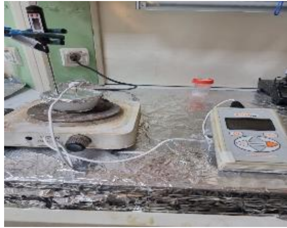
Fig. 4. Thermal conductivity measuring device
