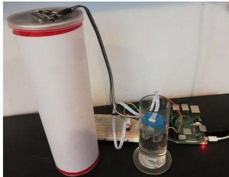
Figure 7. Connection of turbidity and Ultrasonic sensor to Raspberry Pi.
