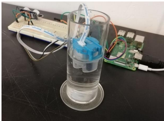
Figure 5. Connection of turbidity sensor to Raspberry Pi.
