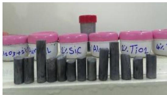
Figure 1. Prepared composite specimens.
