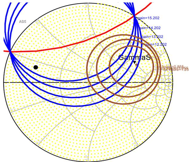
Figure 5. Maximum available gain and minimum NF
