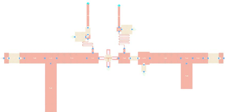
**Figure 9.** The Layout of the LNA with input and output MN
