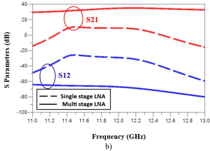
**Figure 12.** S-Parameter Result of Multi-Stage and Single Stage LNA a) Output and Input Return Losses, b) Gain and Isolation Losses
