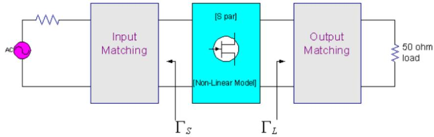
Figure 1. Single stage LNA [11, 12]
