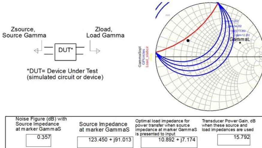
Figure 6. Input and output impedance by load and source pull tool
