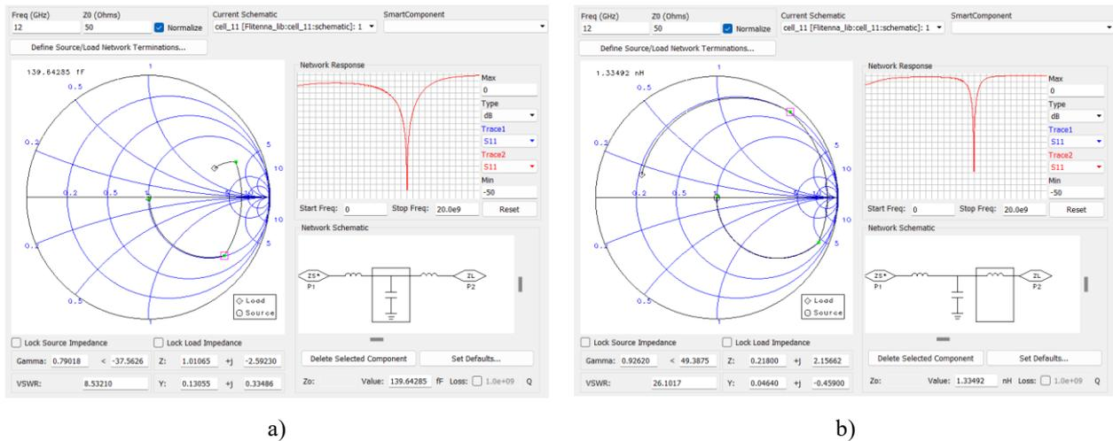
Figure 7. Matching network design, a) IMN, b) OMN
