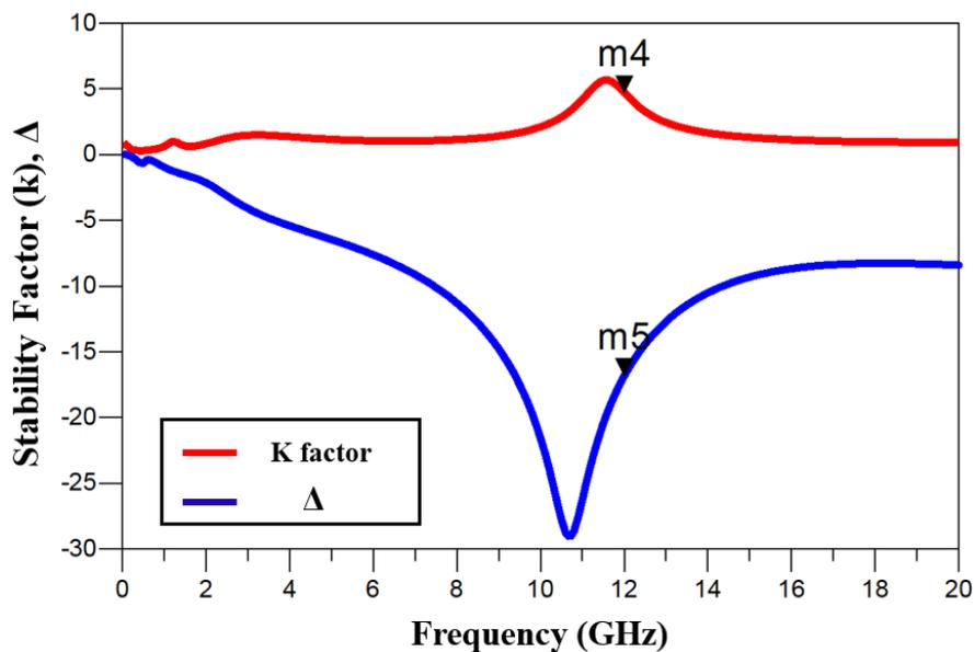
Figure 4. Stability of transistor
