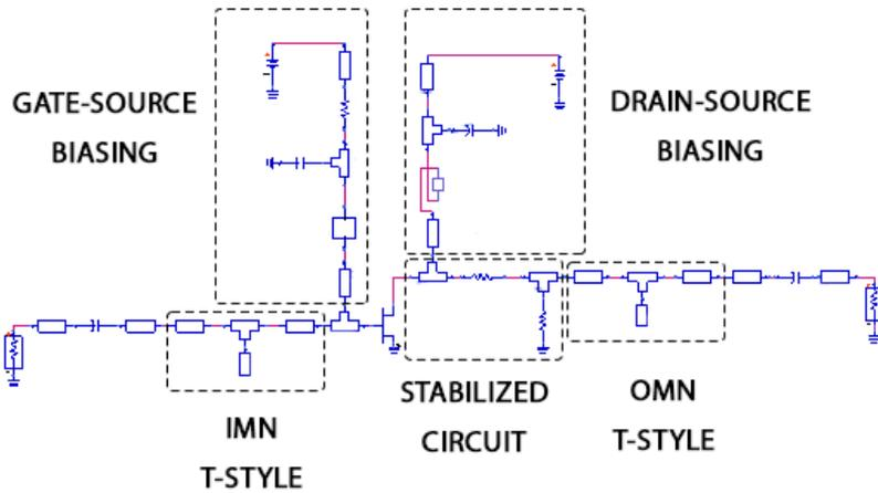
**Figure 8.** The proposed LNA as microstrips
