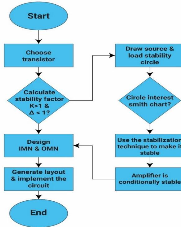
Figure 2. Design steps of LNA
