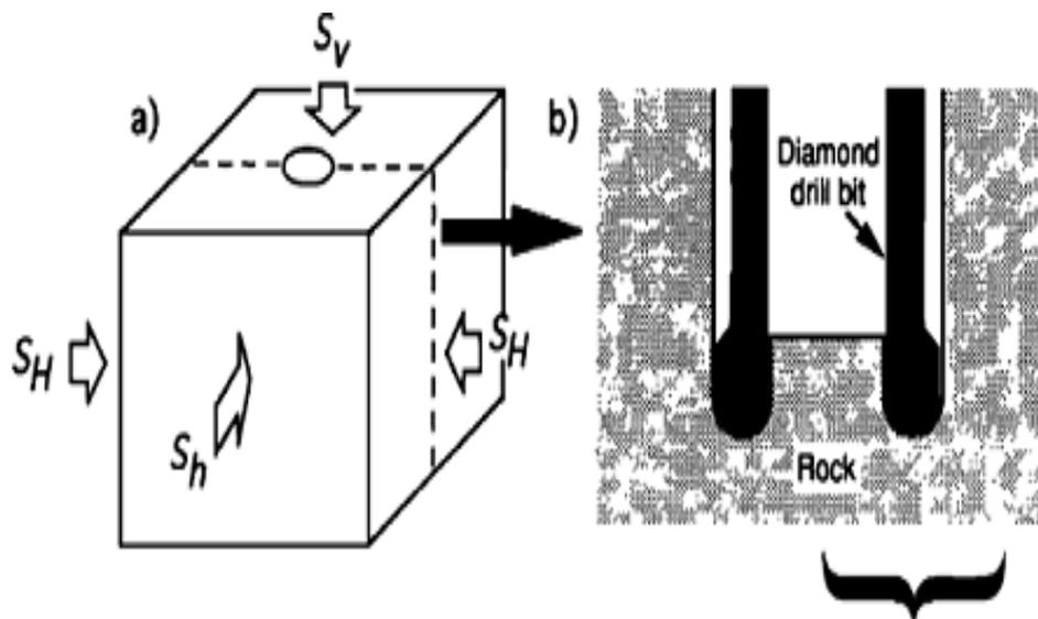
**Figure 1:** A Stress condition of the modelling, B coring with a diamond drill bit [13]
