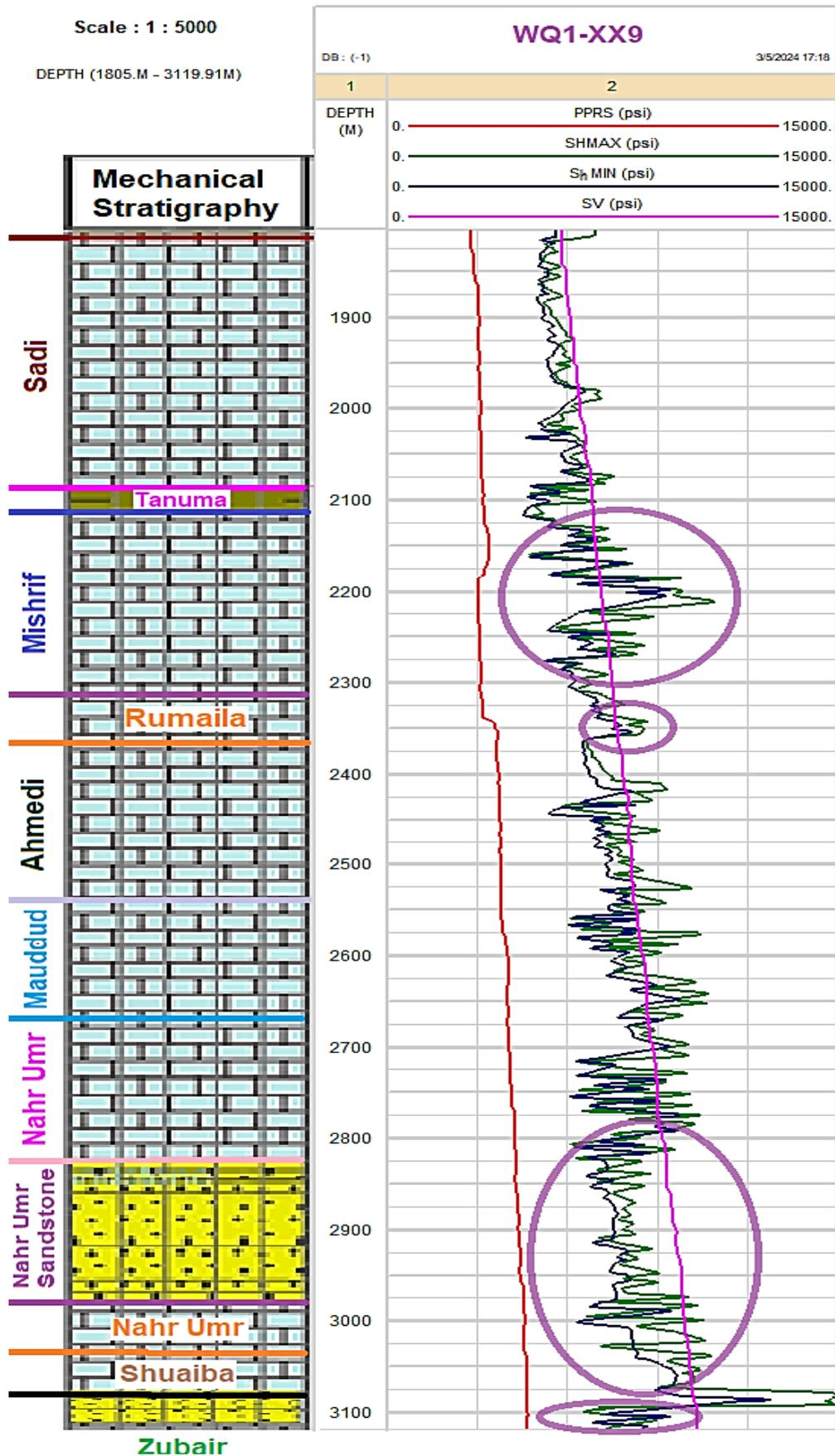
**Figure 14:** Categories of the Well WQ1-XX9 according to the maximum and minimum Stress direction
