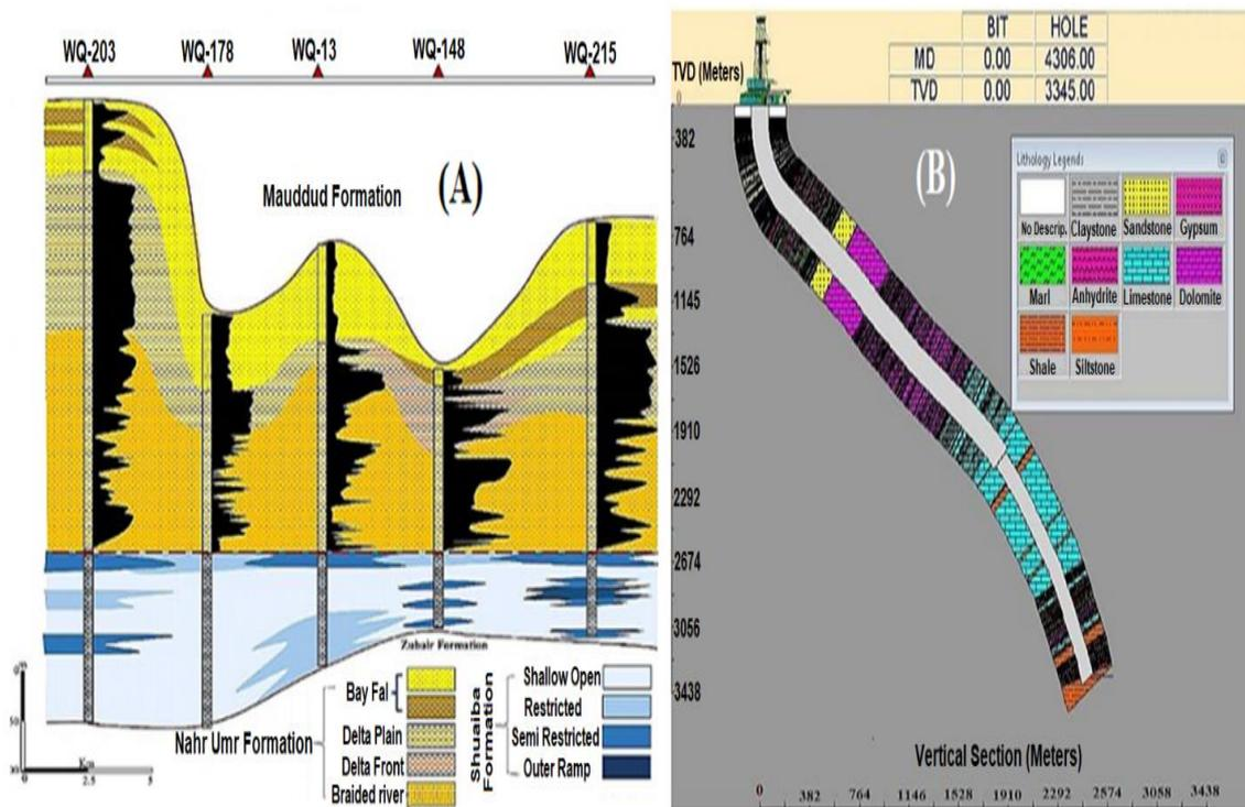
**Figure 3:** A- Cross-section for Zubair Formation in West Qurna oilfield for well WQ1-453 (By researchers) B- Facies changes for Mishrif Formation in the West Qurna oilfield [27]
