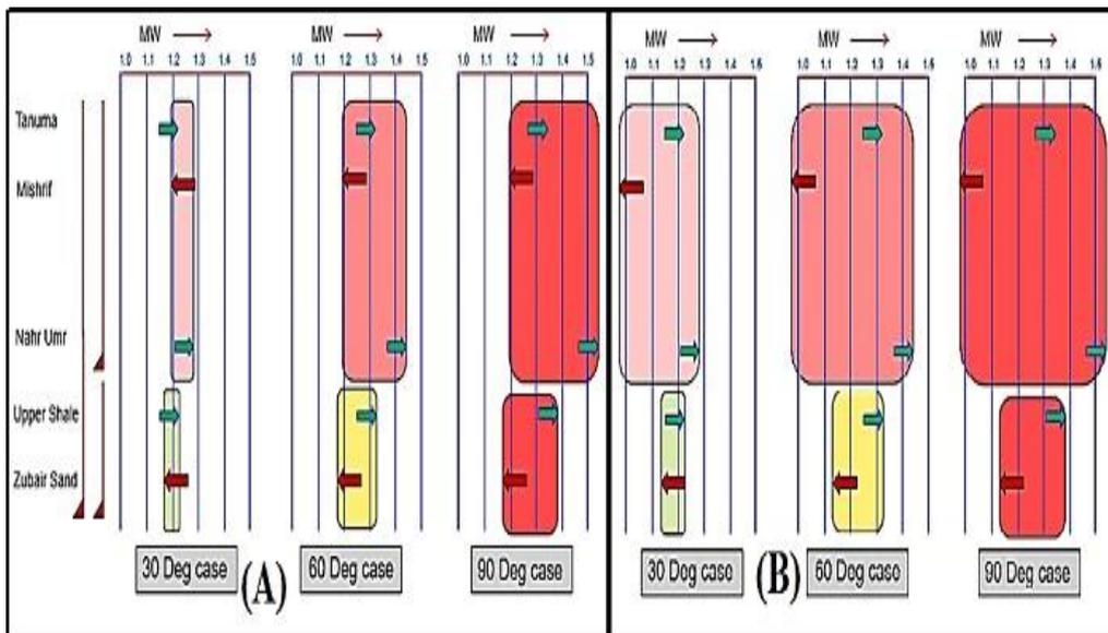
**Figure 10:** Mud Weight differential window for Zubair Formation wells in West Qurna oil field: A-Initial, B- Current phase
