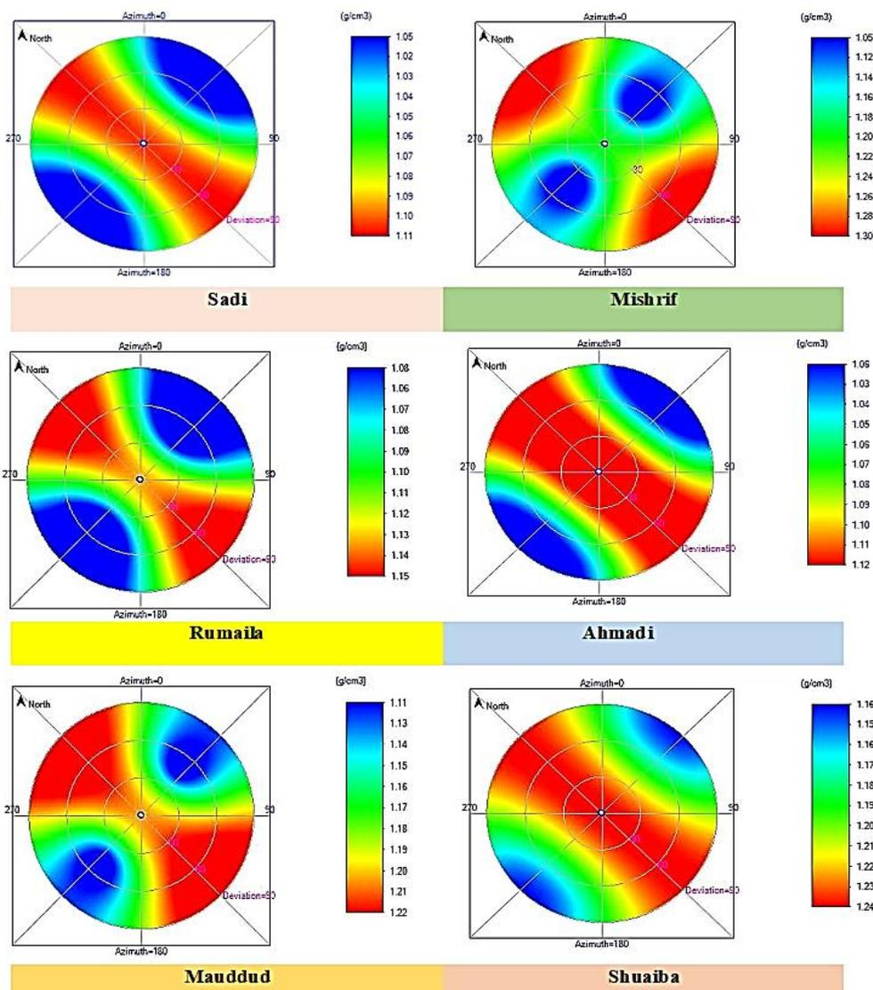
Figure12: WBS plot for regional stress versus mud weight for limestone formations Well WQ1-X56.
