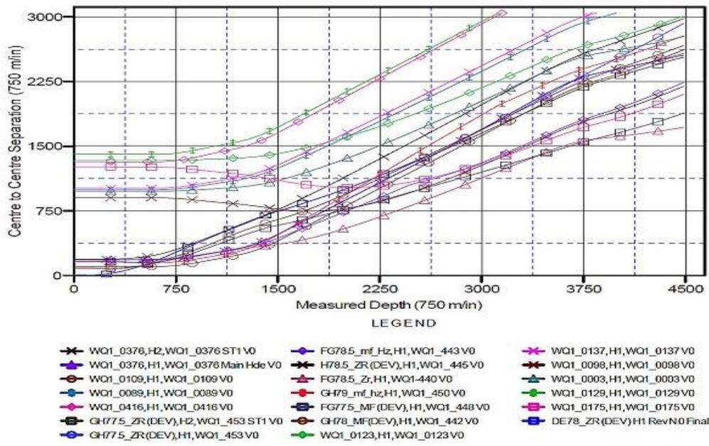
Figure 8: the distance between the wells versus the measured depth
