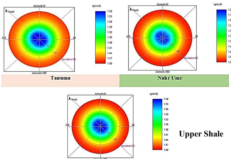
Figure 13: WBS plot for shale formations for Well WQ1-X56.
