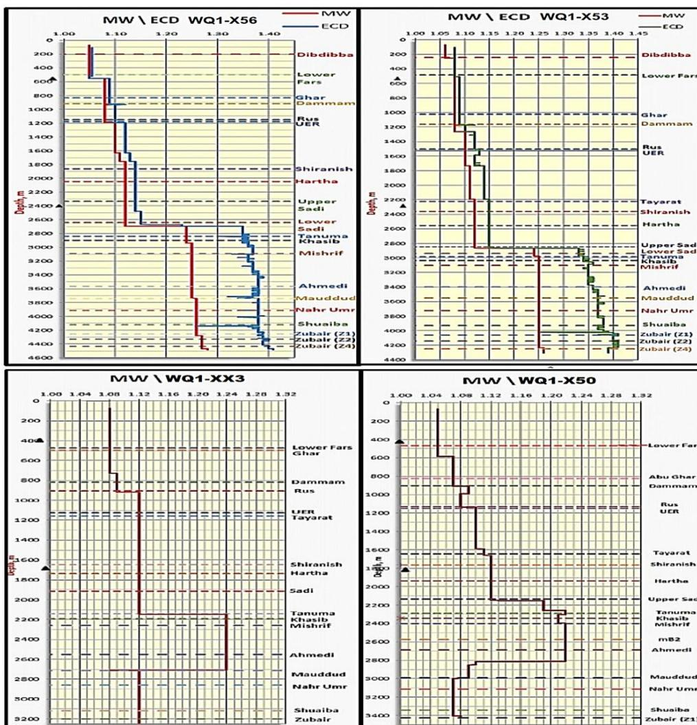
**Figure 11:** Mud weight and ECD (gm/cm<sup>3</sup>) versus depth for wells WQ1-X53, WQ1-X56 (Zubair Formation) and mud weight (gm/cm<sup>3</sup>) versus depth for wells WQ1-XX3, WQ1-X50 (Mishrif Formation)
