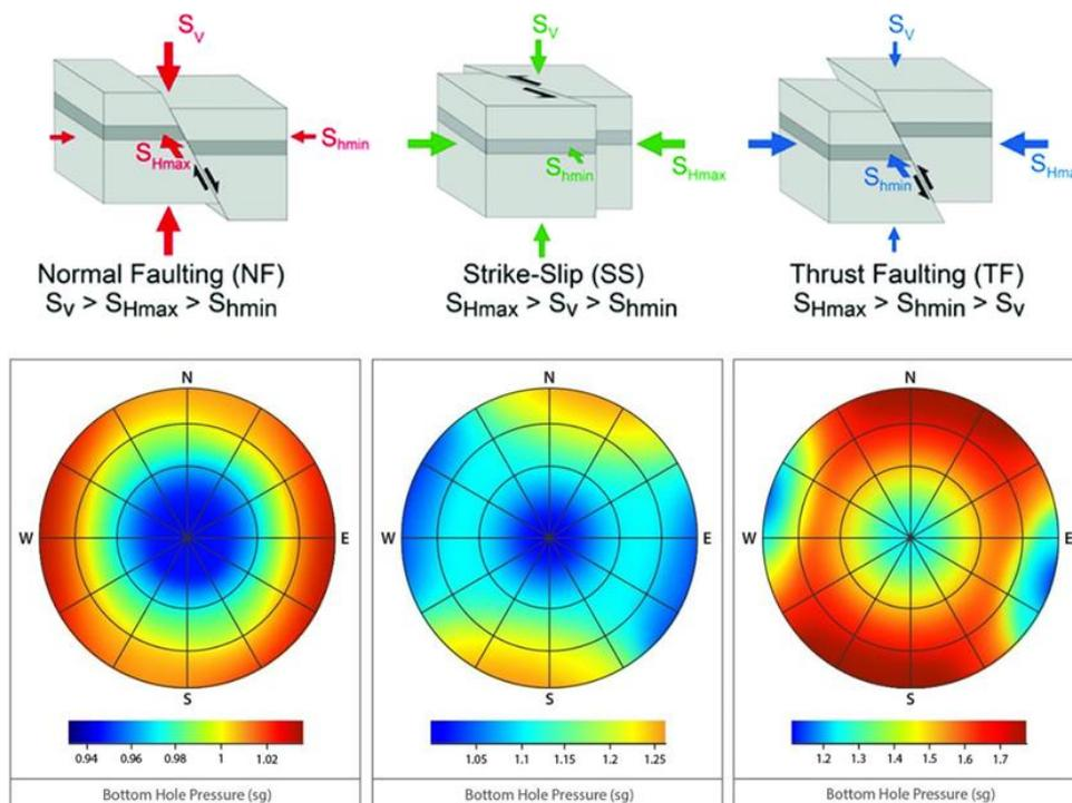
**Figure 4:** Fault system, stress regimes, Breakout development, and borehole stability
