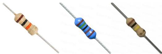
Figure 17. Resistors that limit the current that can pass through an electrical circuit.
