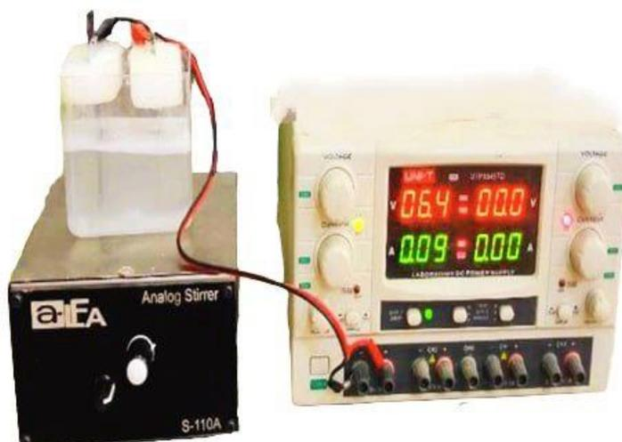
**Figure 1.1 Electrochemical cell system**
