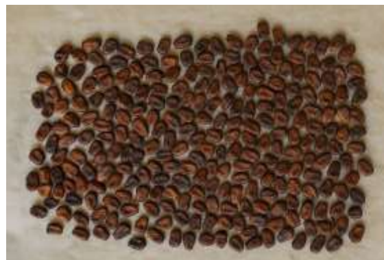
Figure 2: After drying the corn in oven at 115 °C for 8 hours.
