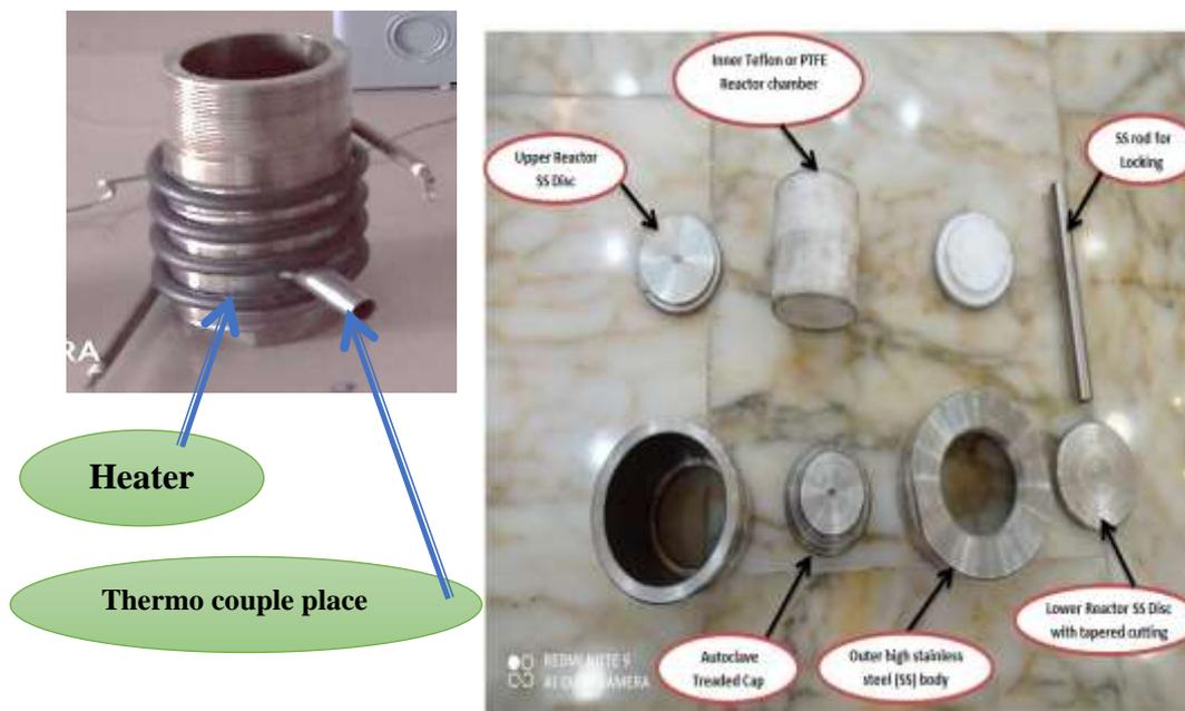
**Figure 2 b:** The different parts of the stainless steel autoclave.
