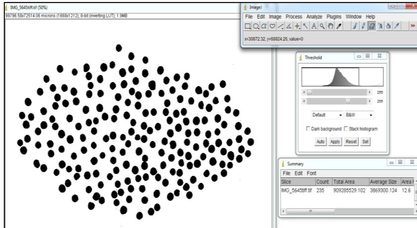
Fig. 2 Analysing the zeolite particles using ImageJ software.
