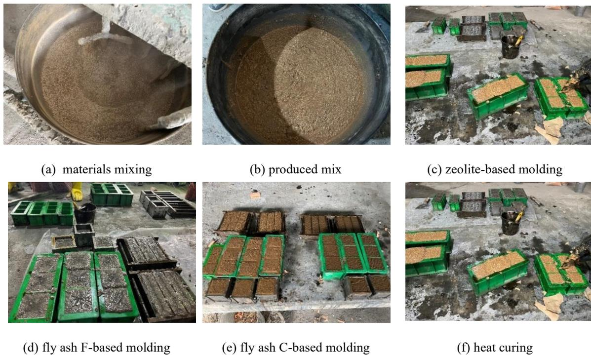
**Fig. 4 Stages of mixing, molding and curing of investigated mixes**
