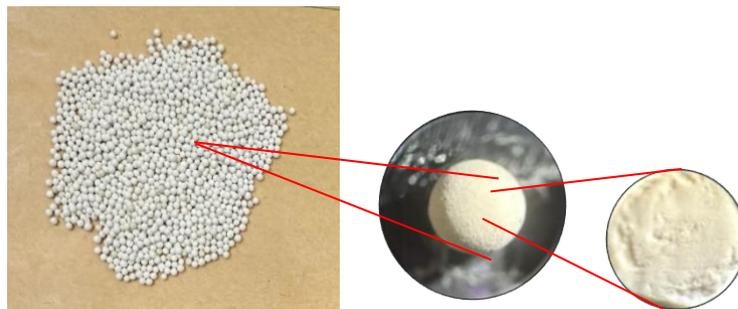
Fig. 1 Waste particles of zeolite molecular sieve used
