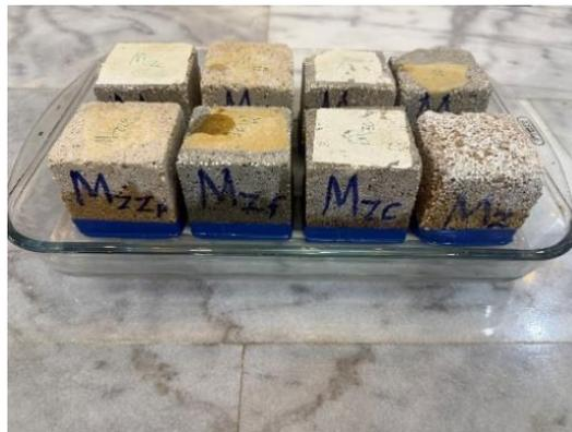
Fig. 5 Sorptivity test
