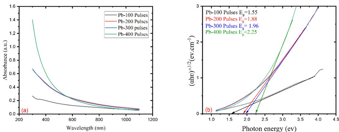
Fig.3. UV-Visible spectra of prepared nanoparticles of Lead oxide at different number of laser pulses. (a) absorbance spectra, (b) Plot of  $(\alpha h\nu)^{1/2}$  versus  $h\nu$  to determine the energy band gap corresponding to indirect transitions.
