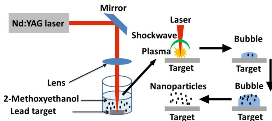
Fig. 1. Setup of the ablation process[11], [12]
