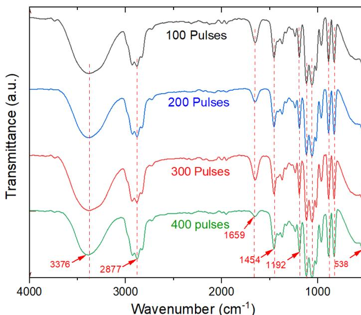
Fig.2. FT –IR spectra of prepared lead oxide nanoparticles.
