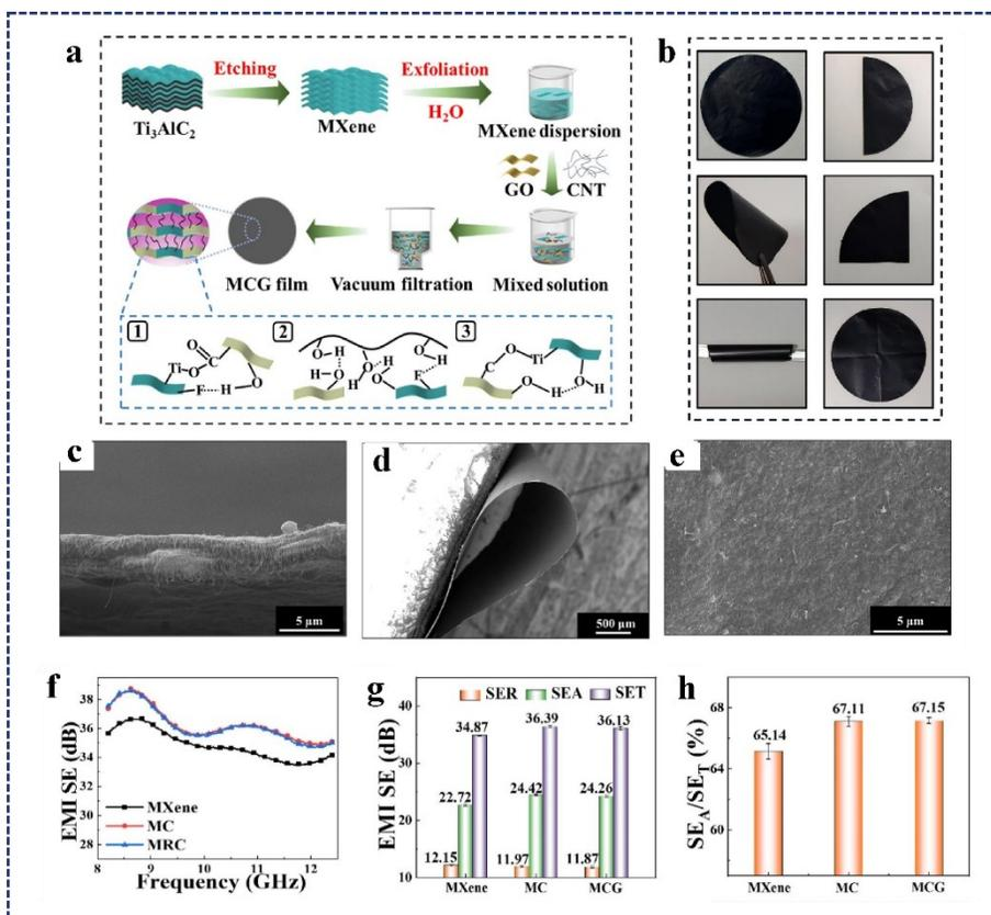
Fig. 5. (a) Schematic diagram of the fabrication of MCG film, (b) Digital photographs of the original MCG film and the MCG film after bending, folding, and rolling, the (c) cross-section, (d) bent, and (e) surface SEM images of the MCG film, (f) EMI shielding performance of the films at different frequencies, (g)  $\text{SE}_A$ ,  $\text{SE}_R$  and  $\text{SE}_T$  values of the films, (h)  $\text{SE}_A/\text{SE}_T$  ratios of the films[41], Copyright 2023, Elsevier Inc.
