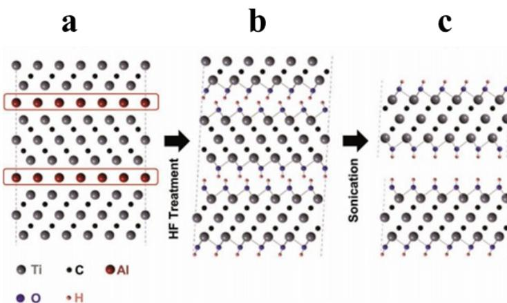
Fig. 1. Schematic illustration of the exfoliation process for Ti<sub>3</sub>AlC<sub>2</sub>, (a) The crystalline structure of pristine Ti<sub>3</sub>AlC<sub>2</sub>, (b) Substitution of Al atoms by hydroxyl groups via selective etching with HF, (c) Separation of MXene nanosheets through ultrasonic cleavage of hydrogen bonds in methanol medium [8], Copyright 2011, WILEY-VCH Verlag GmbH & Co. KGaA, Weinheim
