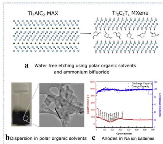
Fig. 2. (a) Selective chemical etching via polar aprotic solvents and ammonium hydrogen fluoride (NH<sub>4</sub>HF<sub>2</sub>) under water-free conditions, (b) Colloidal dispersion and stable suspension preparation through ultrasonic-assisted processing in polar solvents, (c) Integration of electrode components as high-capacity anode materials in sodium-ion batteries [24], Copyright 2020, Elsevier Inc.
