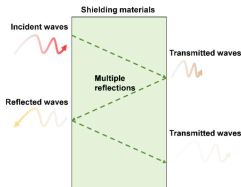
Fig. 3. The shielding mechanism of shielding materials
