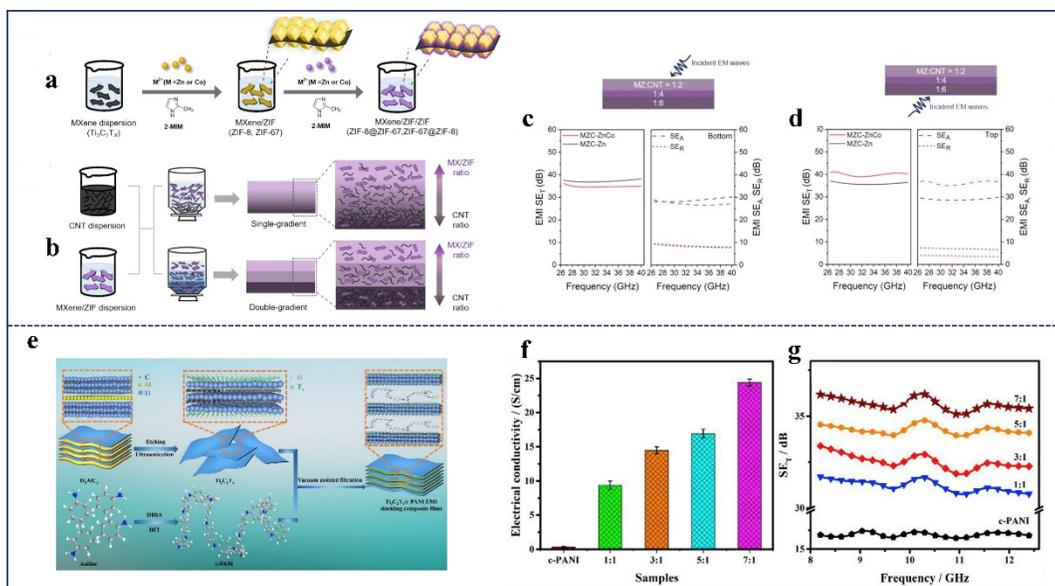
Fig. 4. (a) Schematic diagram of the synthesis of MXene/ZIF, (b) Gradient-structured MXene/MOF/CNF for absorption-enhanced electromagnetic interference shielding, (c, d) EMI shielding effectiveness of MZC-Zn and MZC-ZnCo measured from the (c) top and (d) bottom [34], Copyright 2024, Elsevier Inc. (e) Fabrication of the  $Ti_3C_2Tx/c$ -PANI films, (f) Electrical conductivity, (g)  $SE_T$  of pure c-PANI film and  $Ti_3C_2Tx/c$ -PANI films[35], Copyright 2019, Elsevier Ltd.
