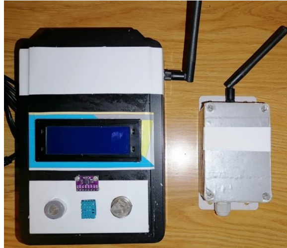
Fig. 1. Enclosure used for the data logger and the wireless units
