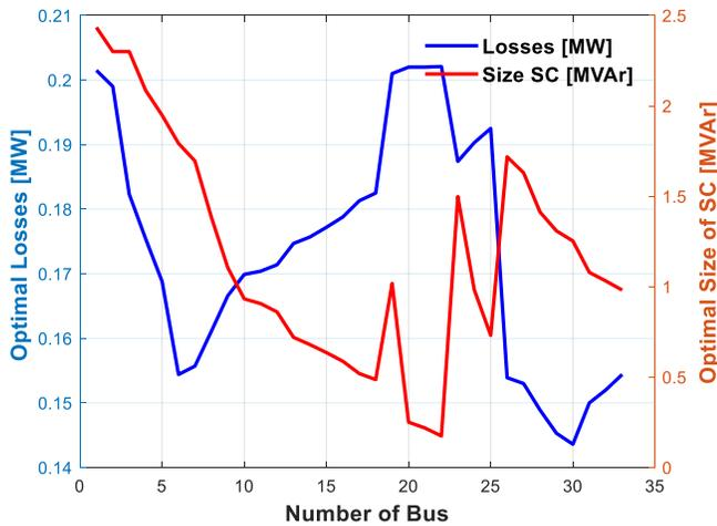
**Figure 5.** The losses of real power [MW] and size of SC [MVar] after installation of SC unit at each bus.
