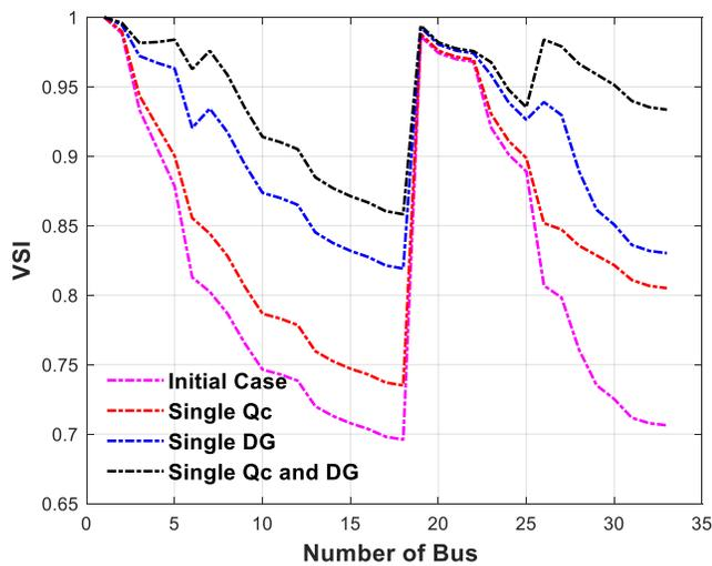
**Figure 9.** Voltage stability index for three cases using GWO.
