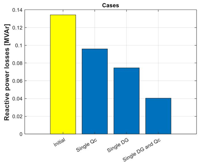
**Figure 11.** Comparison results of reactive power losses.
