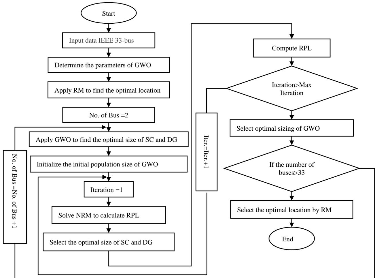
**Figure 3.** Flowchart of proposed approaches on RDN 33-bus.
