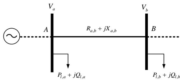
**Figure 1.** The equivalent circuit of RDN.
