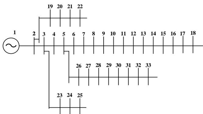
**Figure 4.** Single-line diagram of the IEEE 33 bus power system.
