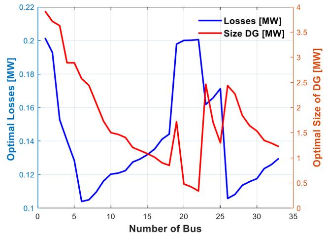
**Figure 6.** The losses of real power [MW] and size of DG [MW] after installing the DG unit at each bus.
