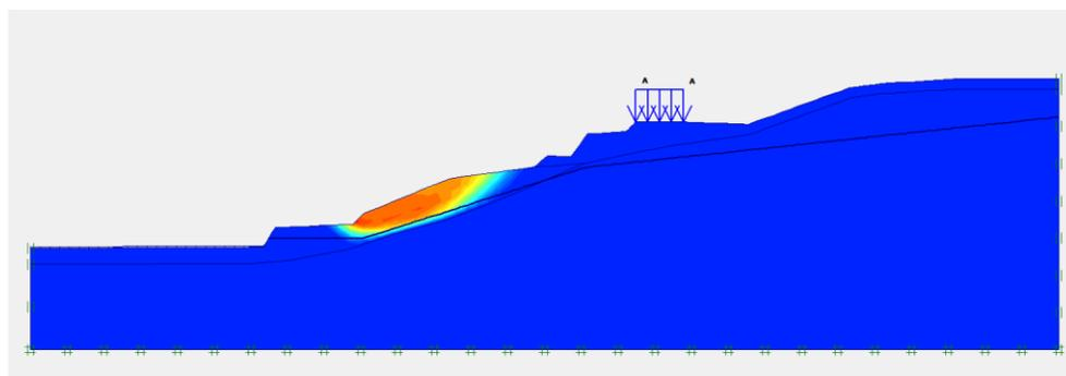
Figure 8. Slip surface in existing conditions
