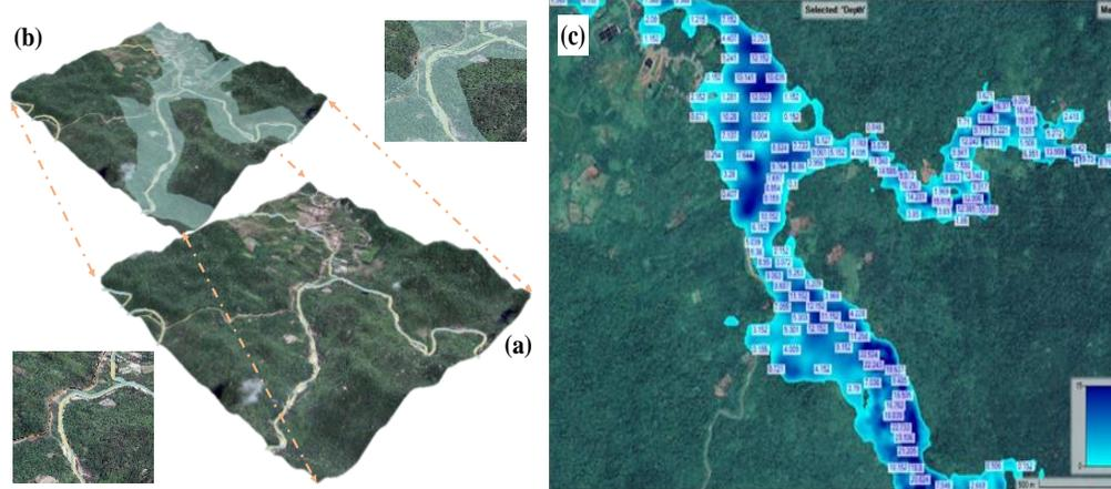
Figure 6. The floodwater level modeling (a,b), ArcScene version 10.8 program, and (c) HEC-RAS program
