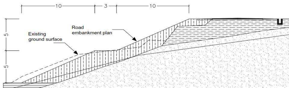
**Figure 4.** Landslide stabilization plan (unit in meters)
