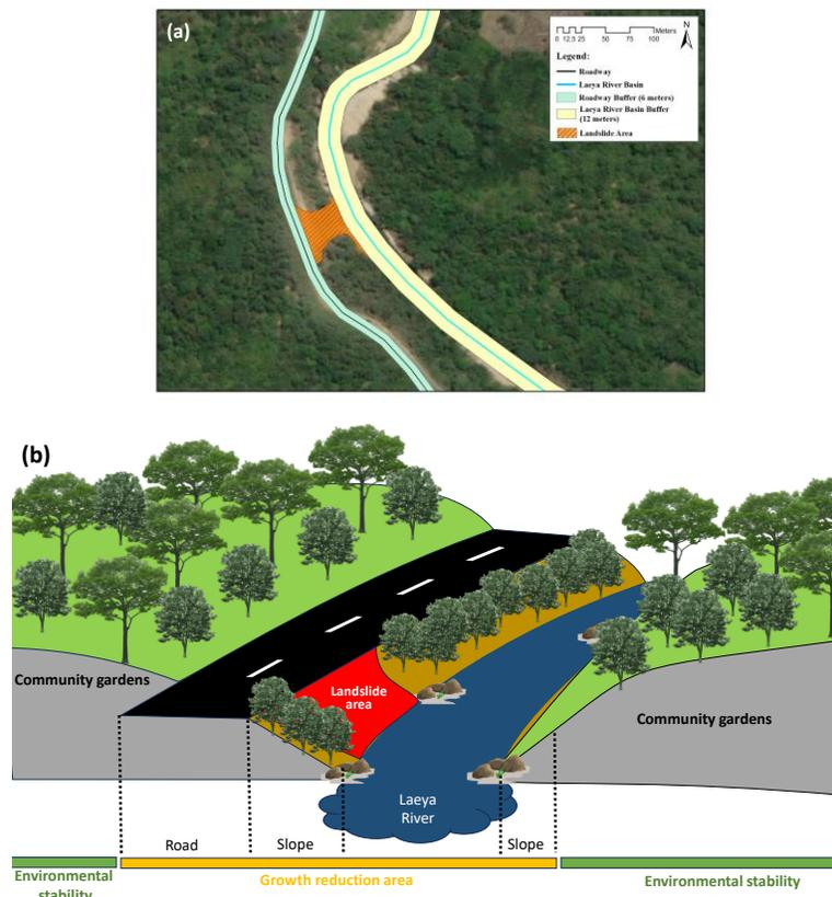
**Figure 5.** Landslide identification (a) Bing satellite imagery, and (b) Theoretical Laeya River cross-section with the affected road
