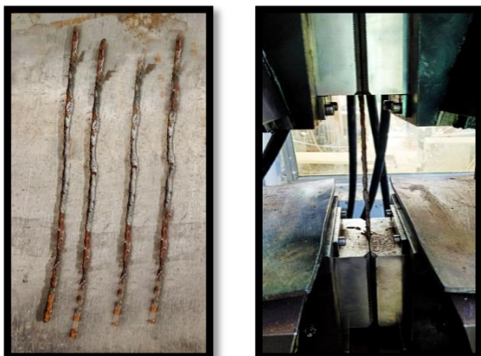
Figure 12 Corroded and non-corroded steel bars tensile test
