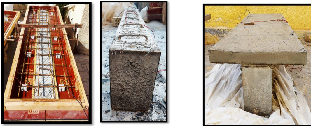
Figure 4 Beam Specimens Cast
