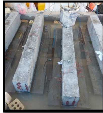
Figure 6 Phases of the corrosion process for first-level specimens
