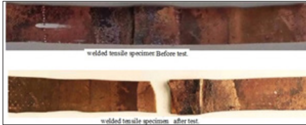
.Figure (8):Broken Tensile specimen after test
