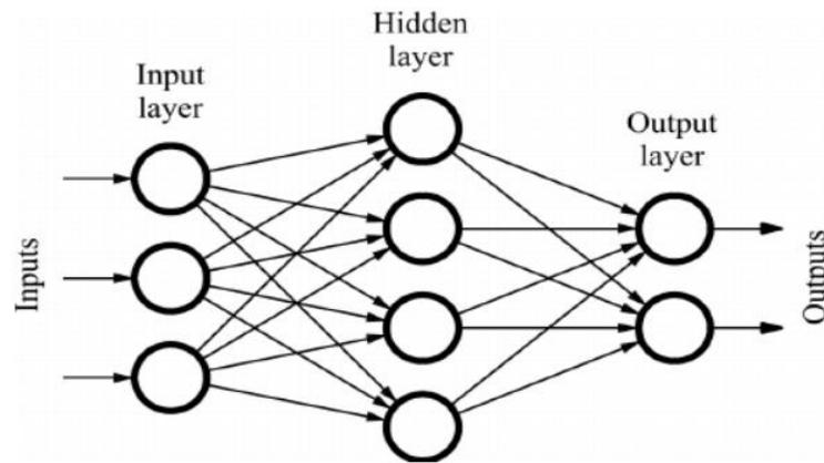
**Figure1: General structure of artificial neural network [3]**
