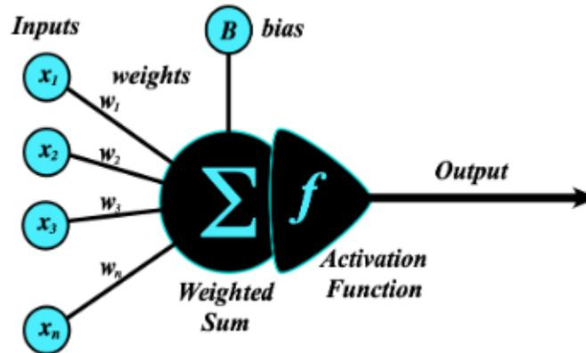
**Figure 3: Weight of each element of the ANN system [4]**
