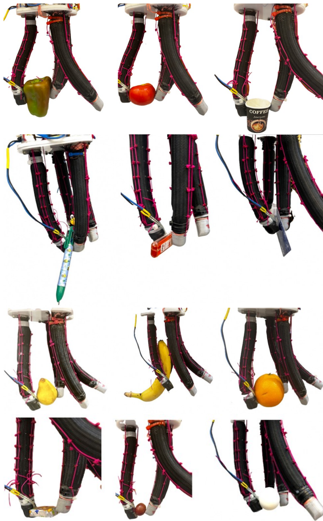
Fig. 24. Handling different types of objects with just two fingers.
