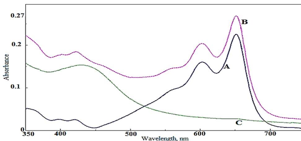
**Fig. 6: Absorbance spectra of 100 $\mu\text{g}$  BH /20 ml treated according to proposed method and measured against (A) reagent blank (B) distilled water and (C) blank measured against distilled water.**
