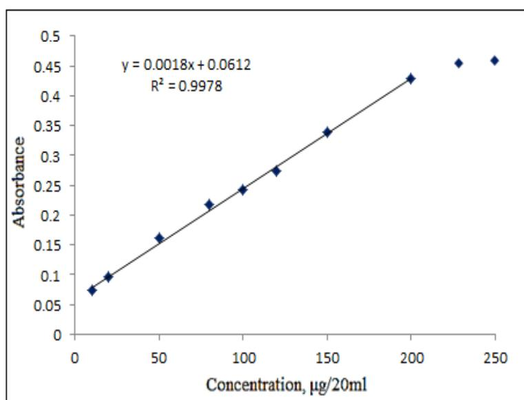
**Fig. 5: Calibration curve for BH determination**
