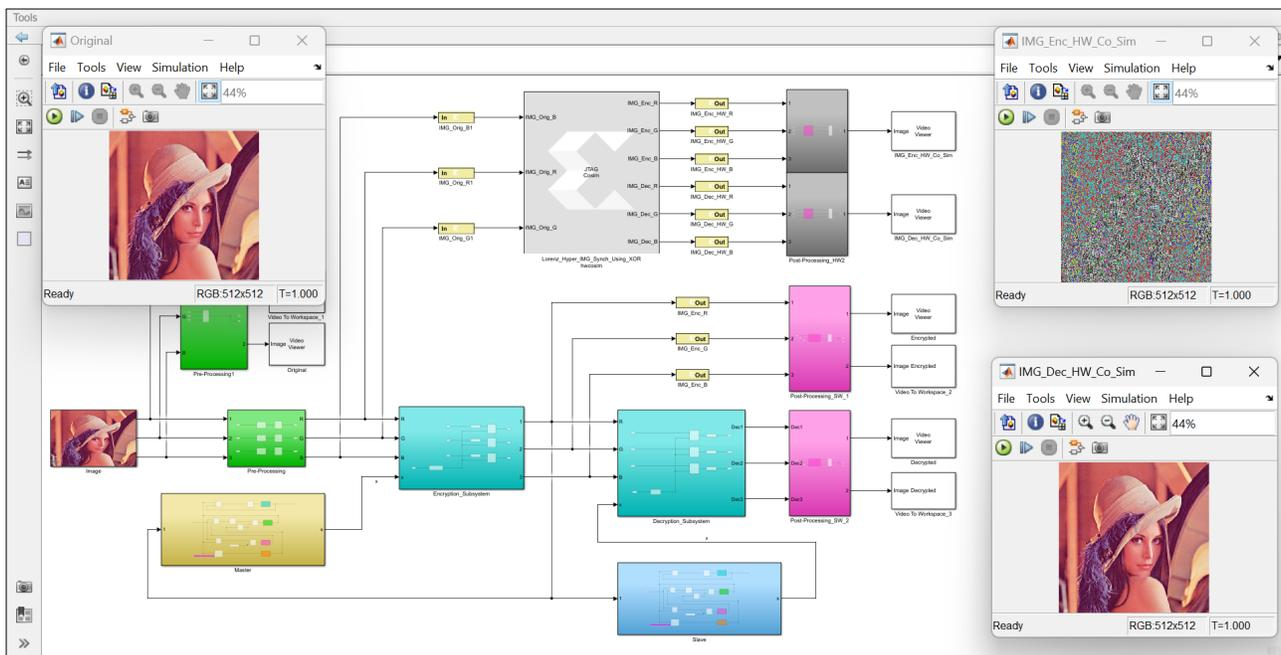
Fig. 8. FPGA hardware co-simulation of the proposed cryptography system using ZedBoard Zynq-7000 FPGA SoC xc7z020-1clg484 development board.
