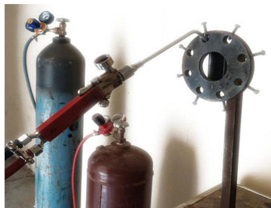
Fig. 1. Illustrate the thermal spray system.
