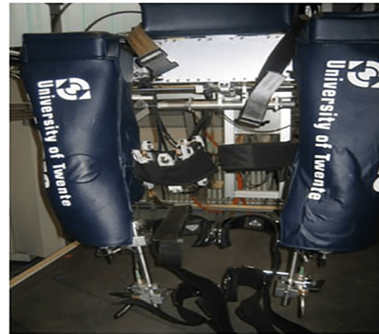
Fig. 21. The sensorized fastening belts and the Lopes exoskeleton for lower-limb rehabilitation [12].
