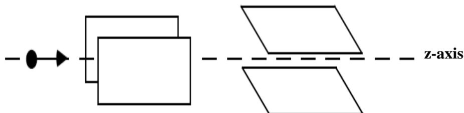
**Fig. 1 : Electrostatic deflector.**
