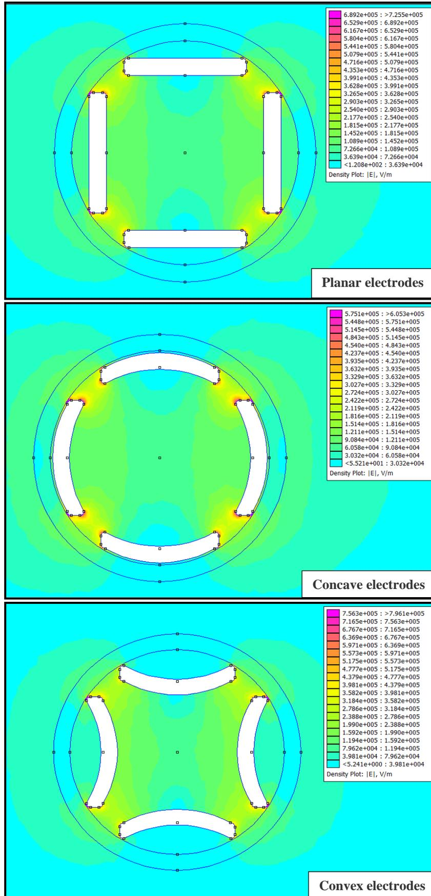
**Fig. 4: The color representation of the magnitude of the electric field intensities  $|E|$  for the designed deflectors.**
