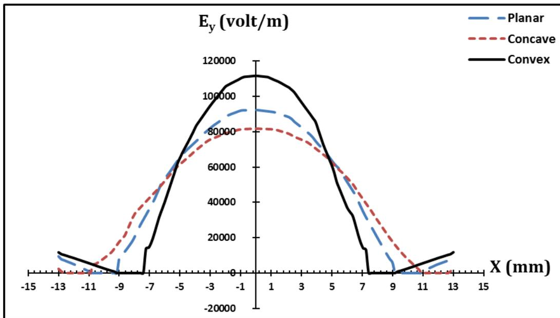
**Fig. 6: Variation of y-direction component of the electric field intensities ( $E_y$ ) with respect to the radial distance ( $X$ ).**
