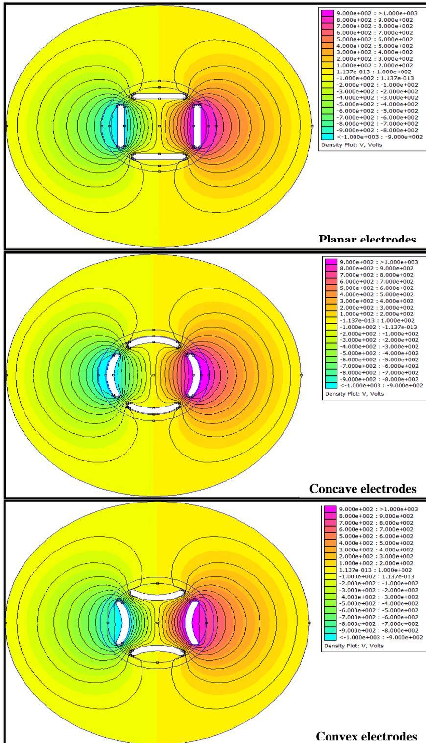
Fig. 3: The color representation of the potential densities mixed with the equipotential lines trajectory ies around the electrodes for the three
