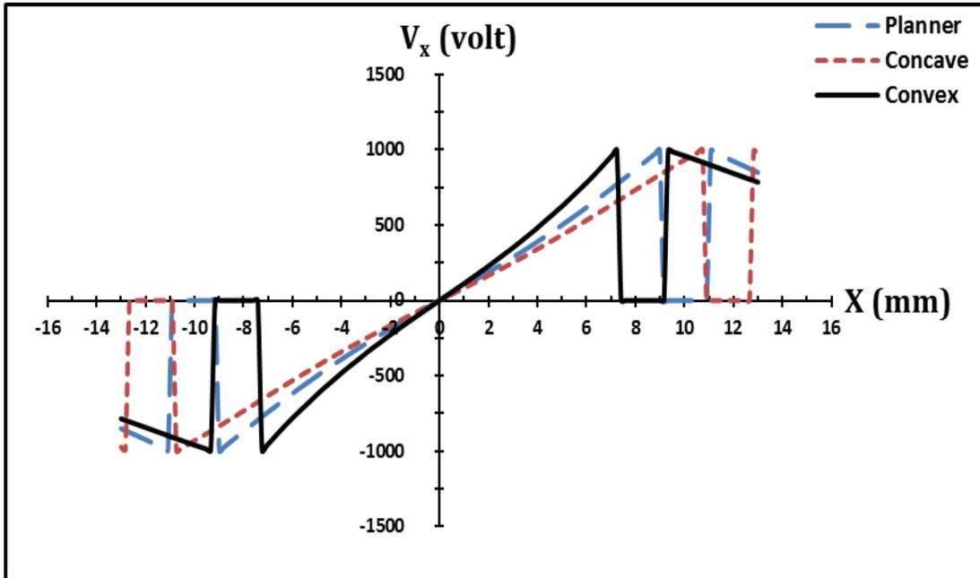
**Fig. 7: Variation of x-direction component of the potential ( $V_x$ ) with respect to the radial distance (X).**
