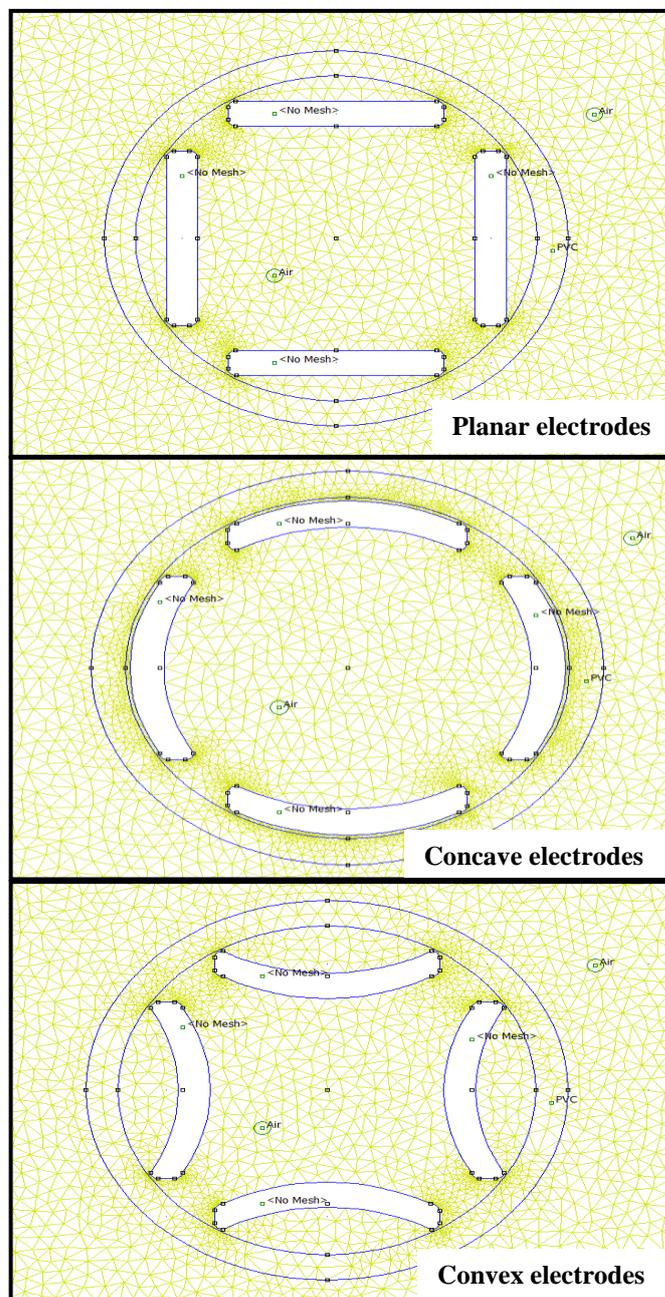
**Fig. 2:** The geometrical shapes of the electrostatic deflectors with the generation of the fine triangular finite element meshes.
