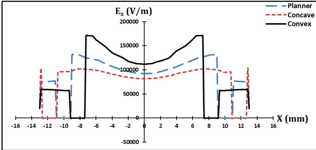
**Fig. 5 : Variation of x-direction component of the electric field intensities ( $E_x$ ) with respect to the radial distance ( $X$ ).**
