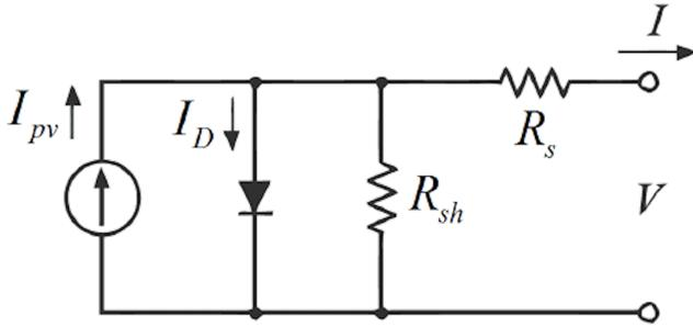
Fig. 1. The equivalent circuit of a PV system
