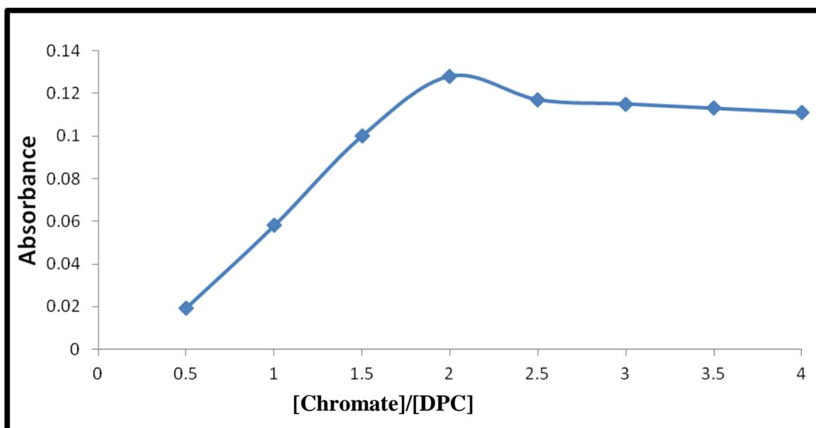
**Fig. 4: Mole ratio plot for chromate-(DPC) reagent complex.**
