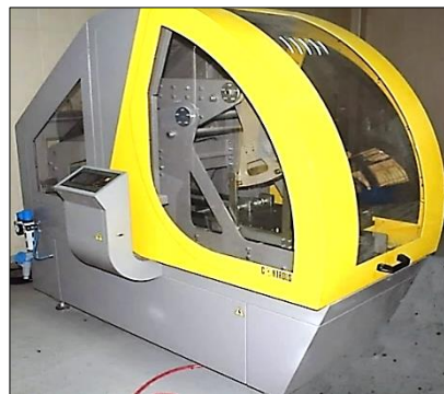
Figure 14. Pneumatic roller compactor
