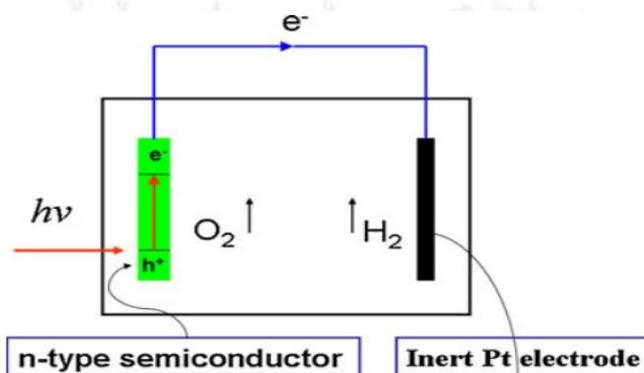
**Fig. 1 Photoelectrochemical Cell Mechanisms: Electron and Hole Dynamics in Hydrogen and Oxygen Gas Generation [8].**
