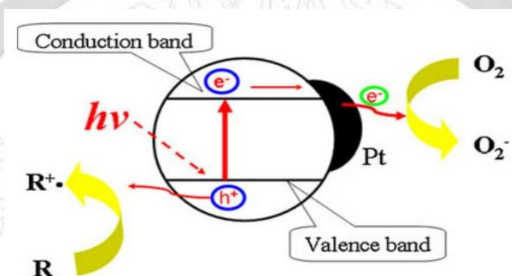
**Fig. 3 Photocatalytic Mechanism of Semiconductors: Electron Dynamics and Reaction Pathways [13].**
