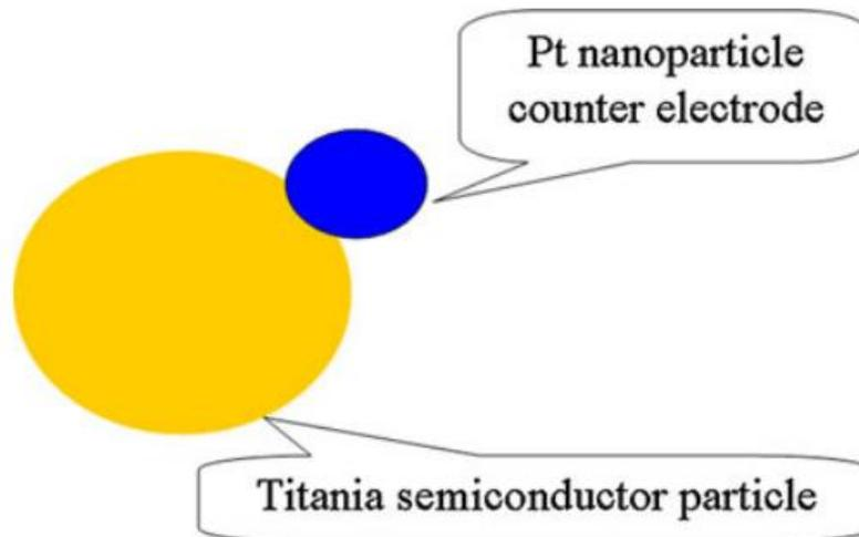
**Fig. 2 Semiconductor Photocatalysts in Aqueous Suspension: A Nanoscale Photoelectrochemical System [12].**
