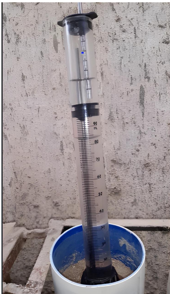
Figure 1. Components of the mini disk infiltrometer
