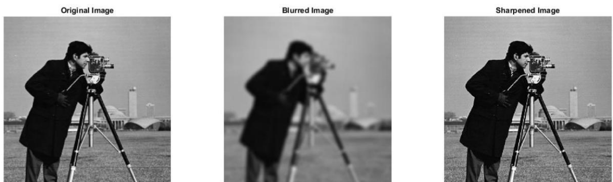
Fig. 8. Performing OFTS (blurred) and OBTS (sharpened) on Cameraman photo
