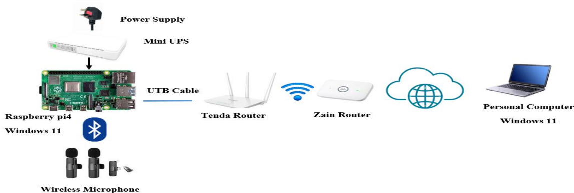
Figure 2: recording Hardware kit diagram for data collection.
