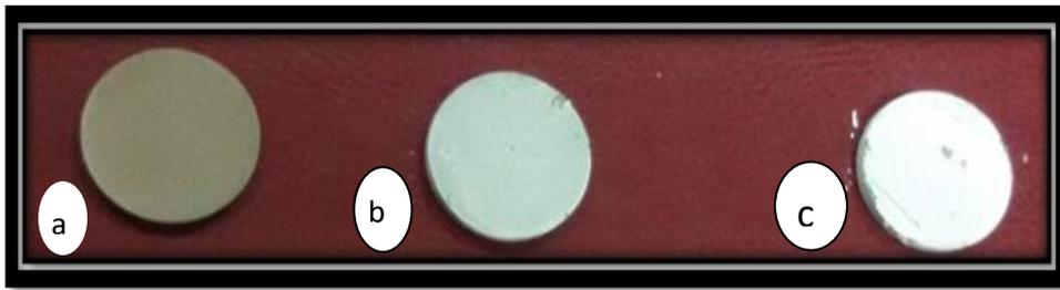
**Figure (1): CP Ti discs (a) Uncoated, (b) nano HA coating, (c) mixture of nano HA &TiO<sub>2</sub>nano HA coating**
