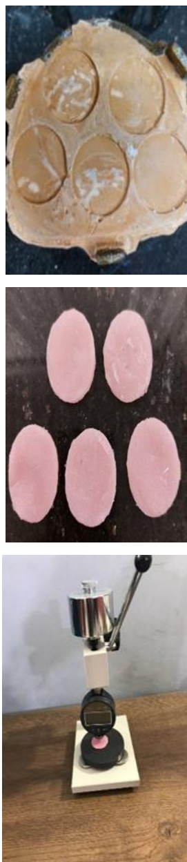
Figure 2: presents the steps of the sample preparation for the Shore A hardness test.
