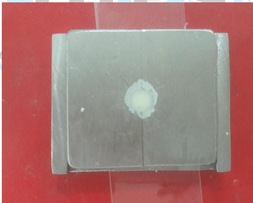
**Figure 2:** Split stainless-steel mold used to prepare specimens for mold for DTS test
