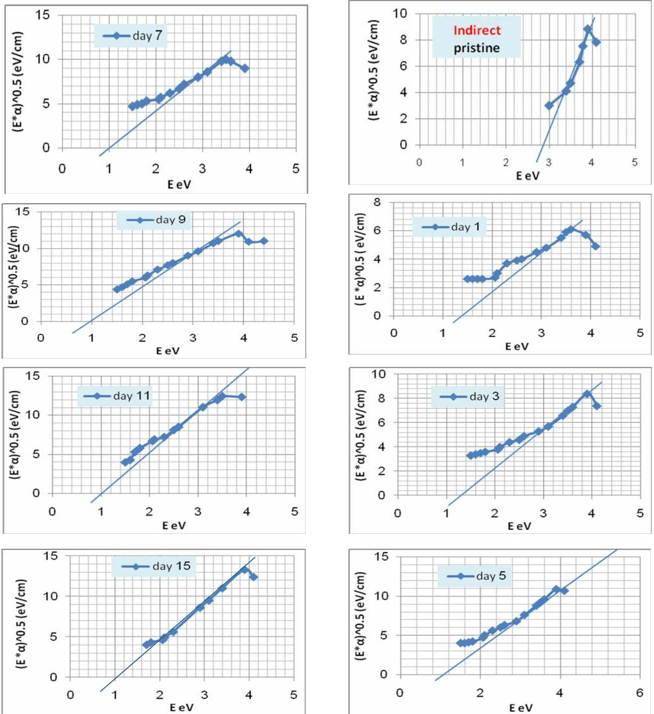
**Fig. 5: The relationship between  $(E \cdot \alpha)^{1/2}$  and the incident photon energy for pristine (not irradiated) and for different exposure time (day).**
