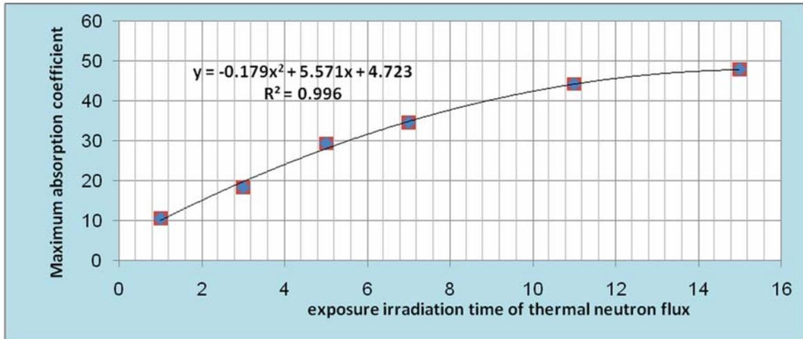
**Fig. 3: The relationship between the maximum absorption coefficient and exposure irradiation time of thermal neutron flux**
