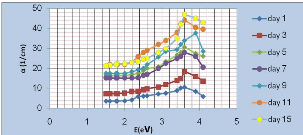
**Fig. 2: The relationship between the absorption coefficient and incident photon energy for exposure irradiation time of thermal neutron flux.**
