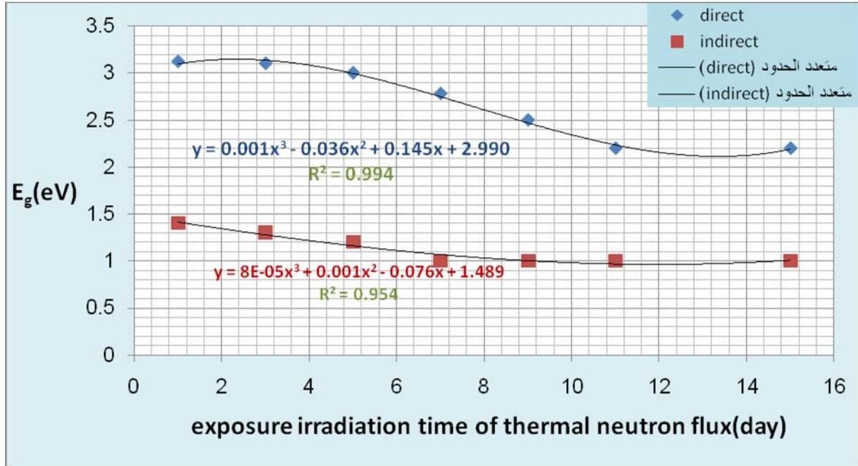
**Fig. 6 : The relationship between band gap energy (eV) and exposure irradiation time of thermal neutron flux.**
