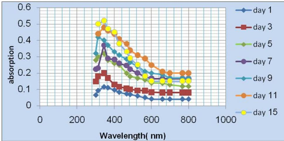
**Fig. 1: UV- visible Spectra of thermal neutron –irradiated CR-39**
