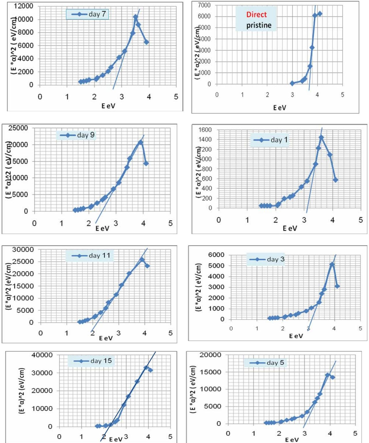
**Fig. 4:** The relationship between  $(E \cdot \alpha)^2$  and the incident photon energy for pristine (not irradiated) and for different exposure time (day).
