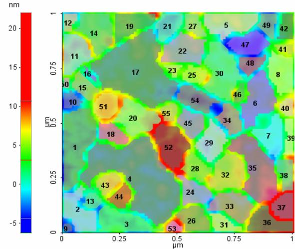
**Fig. 4:** The (3D) nanotopography AFM images of SiO<sub>2</sub> nano film surface annealed at temperature 300°C, RMS surface roughness equal 3.792 nm.
