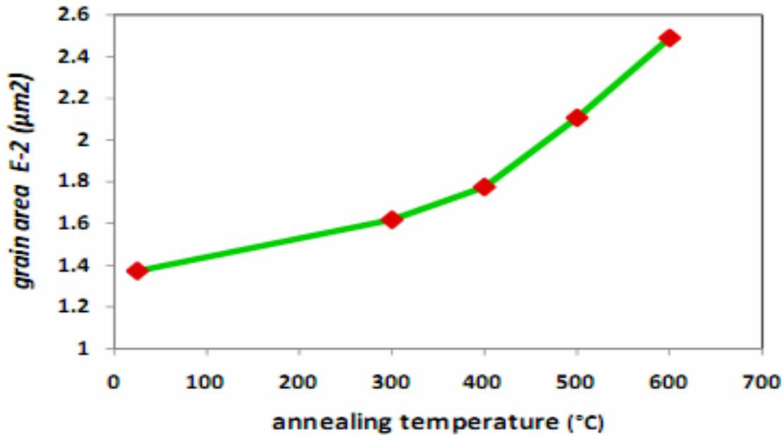
**Fig. 13: The relation between grain area (measured by AFM) and annealing temperature**
