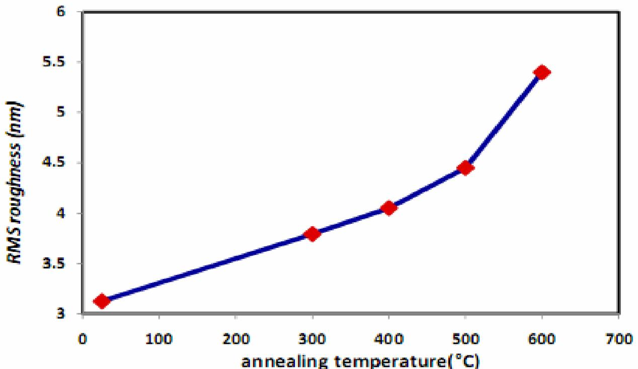
**Fig. 12: Relation between the RMS surface roughness of the SiO<sub>2</sub> nano film (measured by AFM) and annealing temperature.**
