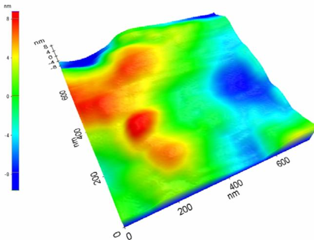
**Fig. 6 : The (3D) nanotopography AFM images of SiO<sub>2</sub> nano film surface annealed at temperature 400°C, RMS surface roughness equal 4.054 nm.**
