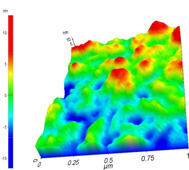
**Fig. 2:** The (3D) nanotopography AFM images of SiO<sub>2</sub> nano film surface, before annealing and RMS surface roughness equal 3.124.nm.
