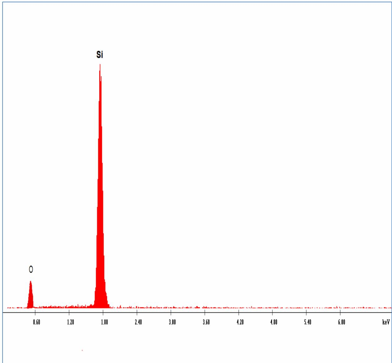
**Fig. 1: Element analysis using (EDAX) of the surface of SiO<sub>2</sub> nano film growth on the surface of Si(100) p-type.**
