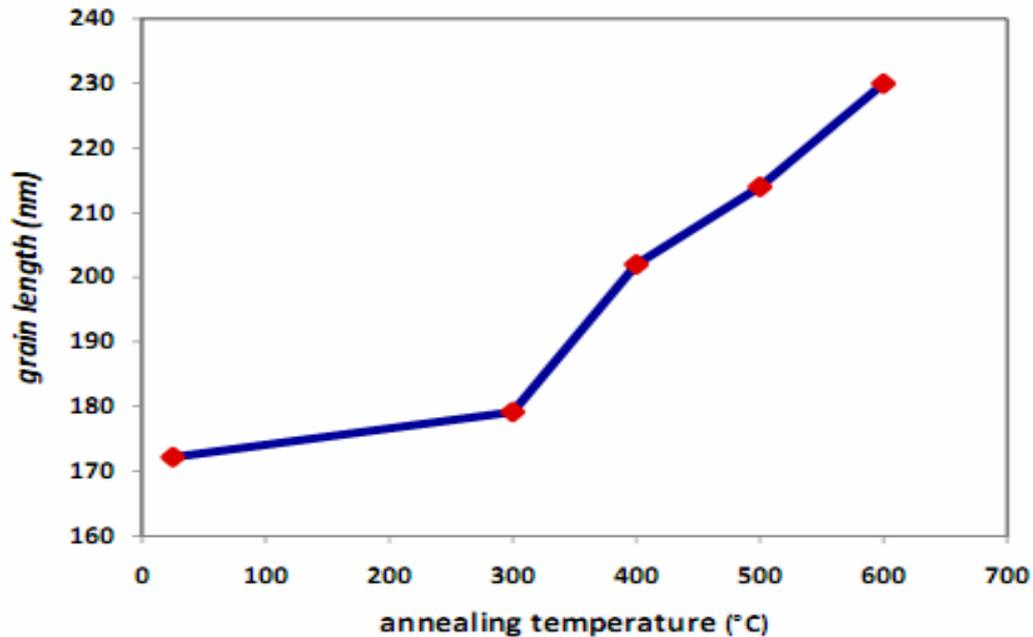
**Fig. 15: The relation between grain length of SiO<sub>2</sub> nano film (measured by AFM) and annealing temperature**
