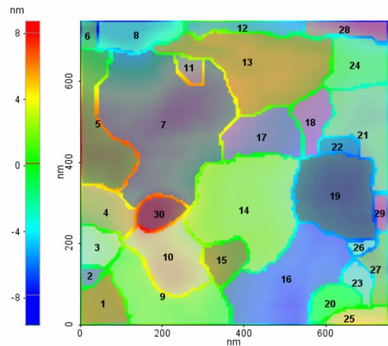
**Fig. 7 : number and distribution of grains on the surface of the SiO<sub>2</sub> which annealed at temperature 400°C measured by using AFM, RMS surface roughness equal 4.054 nm.**
