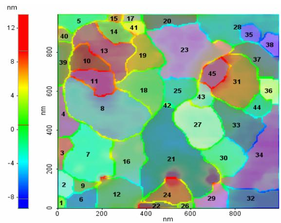
**Fig. 9:** number and distribution of grains on the surface of the SiO<sub>2</sub> which annealed at temperature 500°C measured by using AFM, RMS surface roughness equal 4.543 nm.
