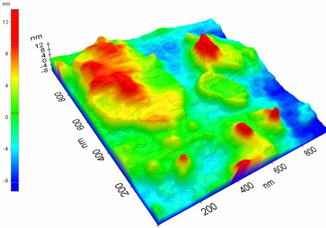
**Fig. 8:** The (3D) nanotopography AFM images of SiO<sub>2</sub> nano film surface annealed at temperature 500°C, RMS surface roughness equal 4. 543 nm.
