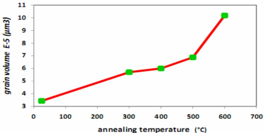
**Fig. 14: The relation between grain volume (measured by AFM) and annealing temperature**
