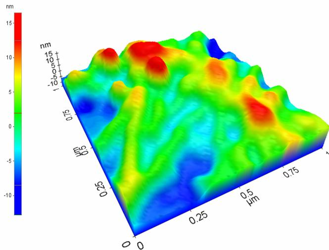
**Fig. 10: The (3D) nanotopography AFM images of SiO<sub>2</sub> nano film surface annealed at temperature 600°C, RMS surface roughness equal 5.482 nm.**
