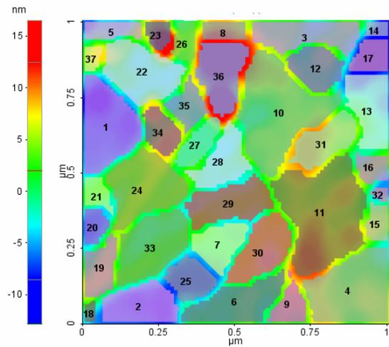
**Fig. 11: Number and distribution of grains on the surface of the SiO<sub>2</sub> which annealed at temperature 600°C measured by using AFM, RMS surface roughness equal 5.482 nm.**
