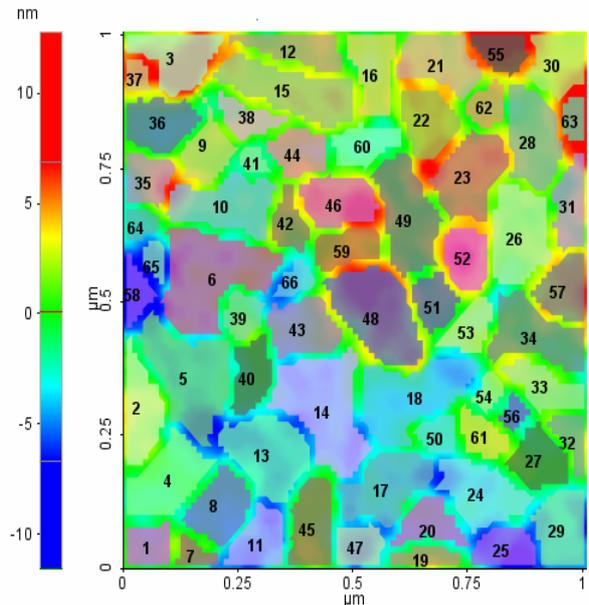
**Fig. 3:** number and distribution of grains on the surface of the SiO<sub>2</sub> before annealing measured by using AFM, RMS surface roughness equal 3.124.nm.
