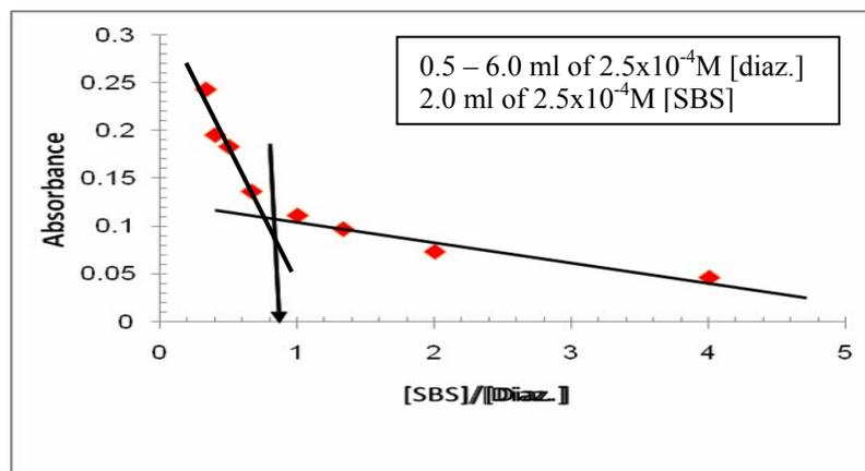
**Fig. 5: Mole ratio method plot**
