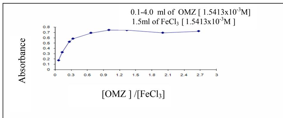
**Fig. 5: Mole ratio plot for OMZ-Fe(III)**
