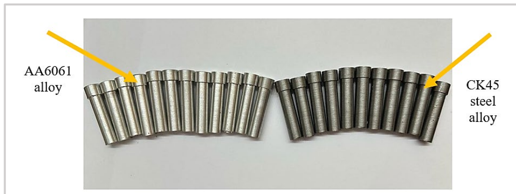
Figure 3: Test pins for two types of metal alloys
