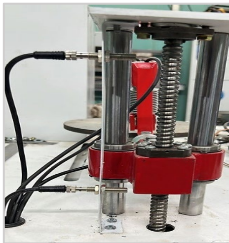
Figure 6: Three shafts for changing an applied load and the load cells fixing
